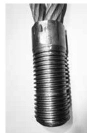
Fig. 38 Damaged thread
